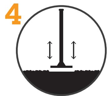
4 Work moisture into clay and compact until firm with tamp. Cover mound clay with conditioner or infield mix.
